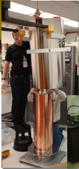
Field compensation magnet for SQUIDs
