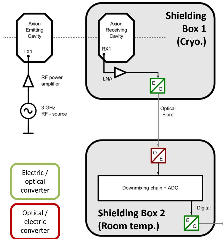
The signal processing electronics can not easily operate at cryogenic temperatures or in strong magnetic fields
