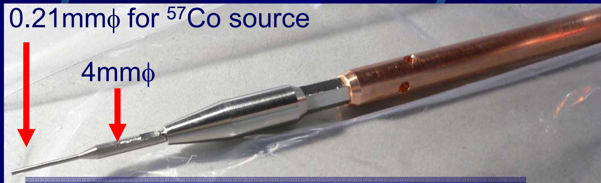
Source rod with a dummy source
