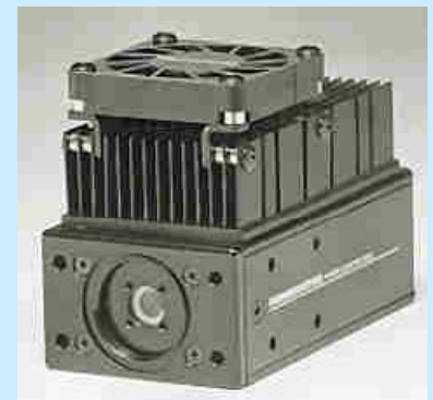
High-QE, low noise, fast PMT module (purchased)
