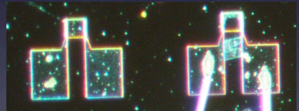
View of two sample sensors: the small (50 \mu\text{m} ) \times (50 \mu\text{m} ) square is the actual TES, and the rectangles are Al contact pads.
